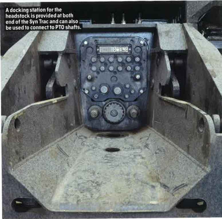
As the vehicle reverses towards the trailer the guide rails on the docking stations slide into position.
