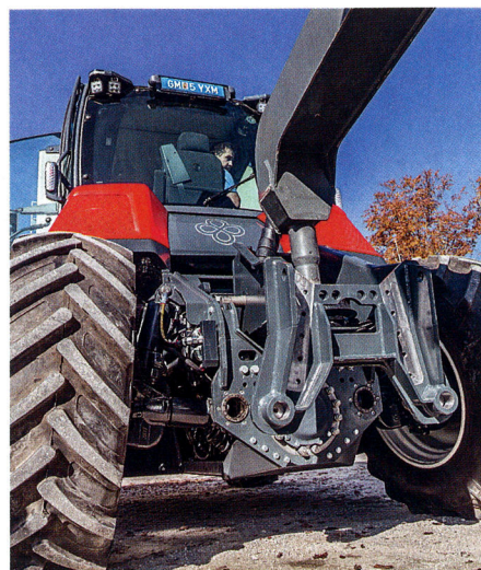
Coupling an attachment starts by lowering the Syn-Trac on its suspension. It's then backed under the implement-side coupler, raised so the two make contact and then the hydraulic clamping system is operated.
